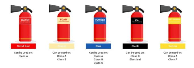
Class A: Combustible, Class B: Flammable liquids, Class C: Flammable gases. Class D: Flammable metals, Electrical: electrical goods, Class F: Cooking oils.
